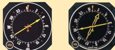
The KI 227-00 (left, above) is the system's non-slaved, standard instrument; the KI 227-01 is a slaved, optional system element. The KR 87 system may also be ordered with a dual-pointer indicator, such as the slaved KI 228-01 indicator (right, above) or the KI 228-00 with a manually rotatable compass card.
